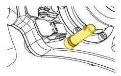
The XS9 Dongle can be easily connected by inserting it into the XS9 interface on the steering wheel.
