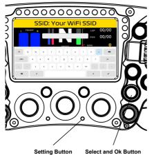
By pressing the Setting button, you can navigate through different menus. You can input the WiFi name and password using the 7-way switch located on the right side.
