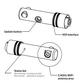
Connect the XS9 Dongle to the steering wheel, and the steering wheel will switch to the PS4/5 dashboard. When the steering wheel is connected to the same WiFi network as the PS4/5, it will be able to retrieve game telemetry data from the PS4/5 via WiFi and display the data on the steering wheel screen.
